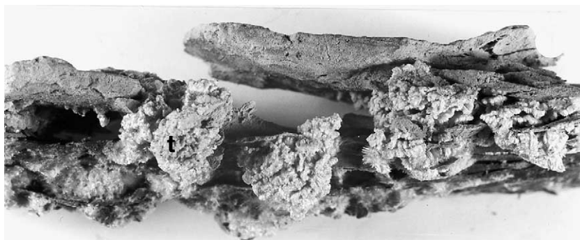
Fig. 6. Roof rock, #26 Colliery, 1-B Mine, spalling in silty shale by crystallizing tamarugite “t”. Westphalian D coal, Sydney Coalfield, Nova Scotia. \times 2 .
