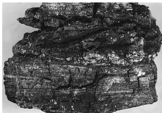
Fig. 2. Oxidizing coal and “sulfur bloom” (white areas) showing oxidation cracks that reduce coal competency. Cantabrian coal, Sydney Coalfield, Nova Scotia. \times 2 .
