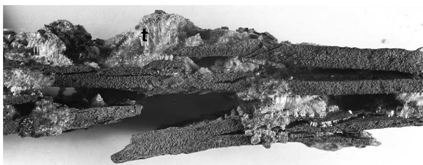
Fig. 7. Roof rock, #26 Colliery, 1-B Mine, showing spalling in silty shale by crystallizing tamarugite “t”. Westphalian D coal, Sydney Coalfield, Nova Scotia. \times 2 .
