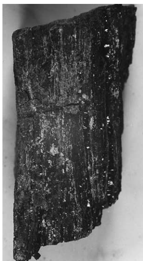
Fig. 3. Coal on which pyritic deposition is outlined by oxidation to hydrated-sulfate minerals (white). Cantabrian coal, Sydney Coalfield, Nova Scotia. \times 2 .
